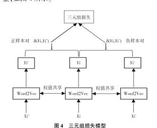
Fig. 4 Model with triplet loss
